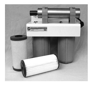
**Series 200 High Flow Drinking Water Systems** provide 3 or 6 gpm of carbon filtered and UV protected water. A two-stage cartridge filtration process removes sediment, treats for taste & odor improvement, and is capable of eliminating high levels of chlorine.
